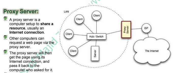
Proxy servers are often used instead of router since additional software can be easily installed on the computer such as anti-virus, web filtering etc.
