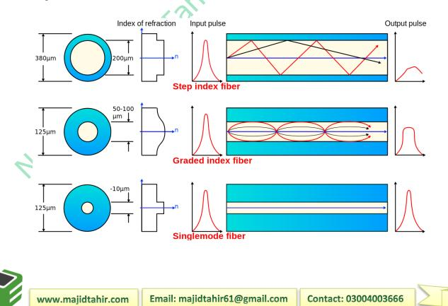
**Fiber optics** is a technology that uses glass (or plastic) threads (fibers) to transmit data. A fiber optic cable consists of a bundle of glass threads, each of which is capable of transmitting messages modulated onto light waves.
