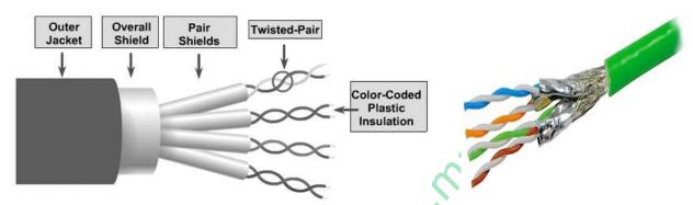
The extra covering in **shielded twisted pair** wiring protects the transmission line from electromagnetic interference leaking into or out of the **cable**. STP cabling often is used in Ethernet networks, especially fast data rate Ethernets. Contrast with UTP.
